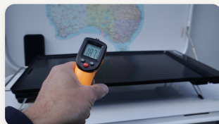
Checking surface temperature — 187°C and climbing
